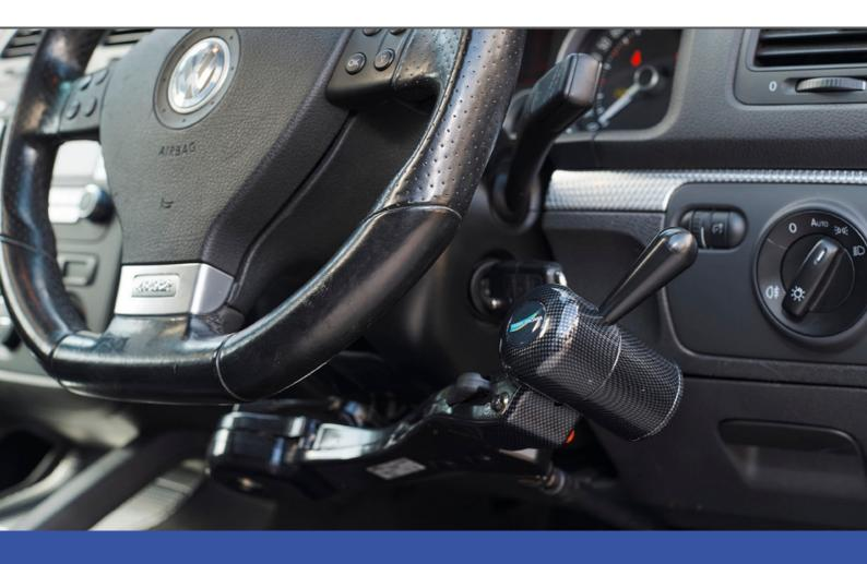
The Ergonomic Radial Accelerator is a quality hand control designed for operation with limited dexterity. The choice of ergonomic palm or lever grip handle coupled with the ability to customise the handle weight and rotation totally personalises the product to the user's individual strengths, preferences and capabilities
