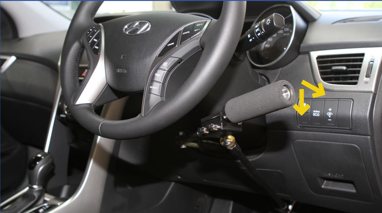
Push-Pull and Push-Pat hand controls for accelerator and brake
