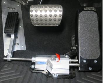
The manual left foot accelerator is designed to be easily released and refitted to accommodate different drivers.
